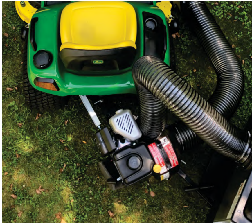
View of Collection Unit sitting to the Right of Operator
